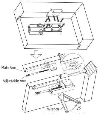
Use spanner to spin the lower square head 45°, parallel the main arm to the door and mount it on the upper square head
